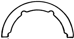
FIG. 69.—Grooves and chamfers.
